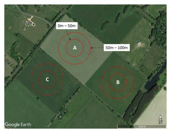
Three survey waypoints are labeled Points A, B, & C, and the two distance bands (0 - 50m and between 50 - 100m) at each point are illustrated.
